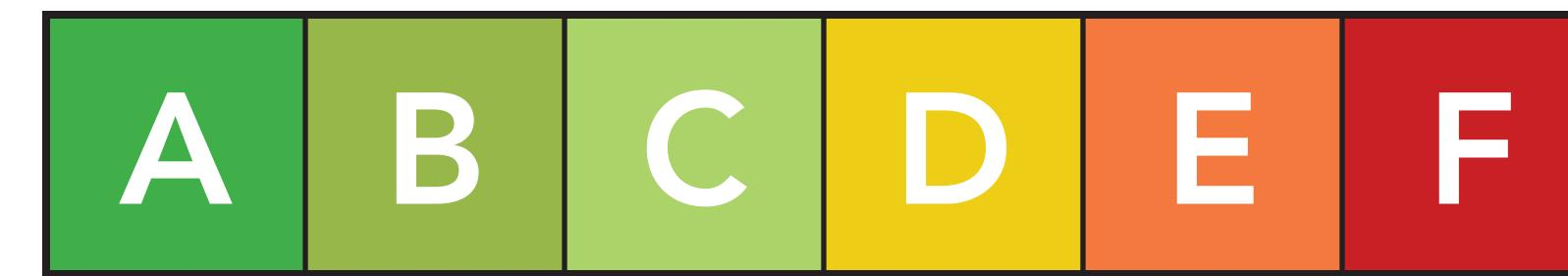
Level of Service describes how smoothly traffic moves by evaluating vehicle delay and speed, using a scale from A to F. Grades A through C indicate generally stable, free-flowing conditions, D and E signal increasing congestion and noticeable delays, and F represents heavily congested, stop-and-go traffic.
